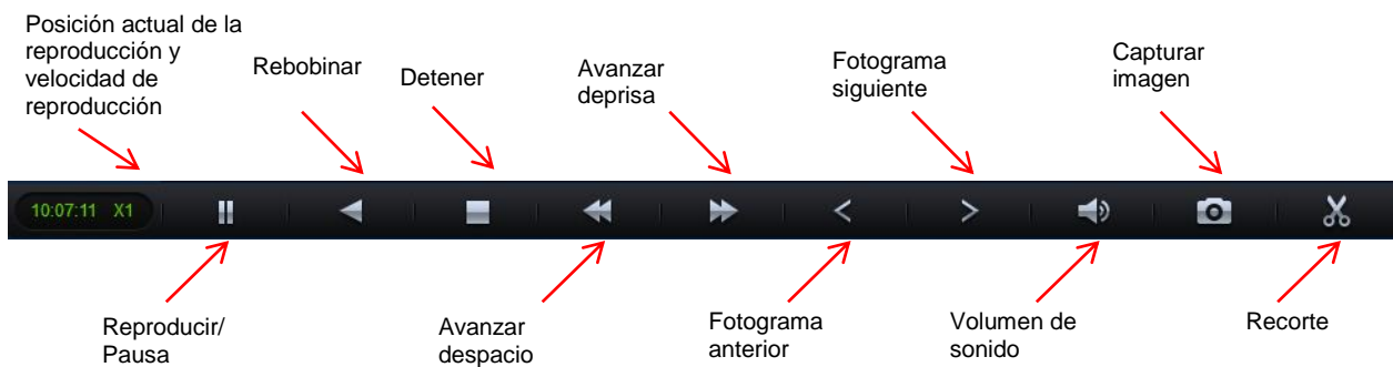
Panel de control del Panel MDR 2.0: Figura 134
